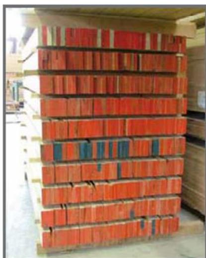
Laminated products are realised with three layers of wood glued with opposing fibres, to compensate for the natural tension present in the structure of the wood and to ensure the stability of doors and windows.
